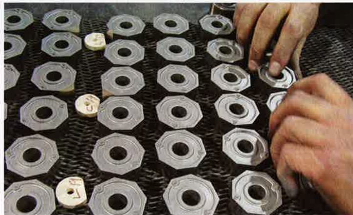
Fig. 3. TempTabs go through continuous furnaces without interrupting production.
